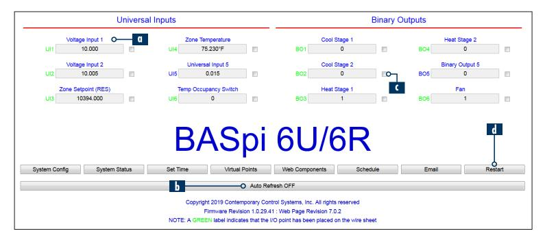
The main web page provides an overview of all real points plus access to other web pages. To configure a point, click on the point name (a) and a configuration page will appear. To observe the updated data for each point, click Auto Refresh button to ON (b). Point values can be temporarily forced by checking the box adjacent to the point
